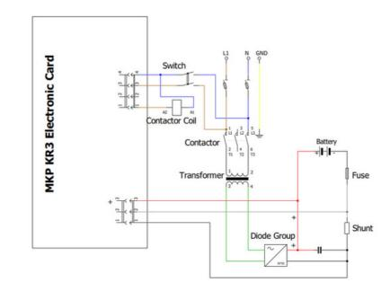
Transformer pin 1 -> 0V Transformer pin 2 -> 230V
