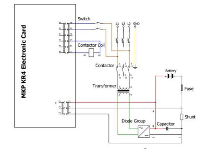
Transformer pin 1 -> 0V Transformer pin 2 -> 400V
