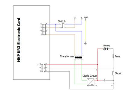
Transformer pin 1 -> 0V Transformer pin 2 -> 230V The warranty period of our products is two (2) years starting from the invoice date.
